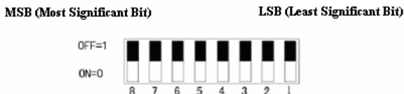
Figure 3-3-3 Binary Value Relationship between Switch Status & Station Address
